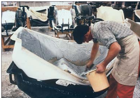
Fig. 16: Manual application of a bonding paste
