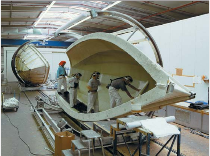
Fig. 20: Manufacture of a boat hull using the hand lay-up technique
