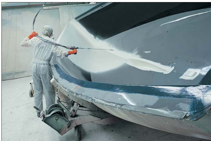
Fig. 15: White gelcoat being sprayed onto a boat mould
