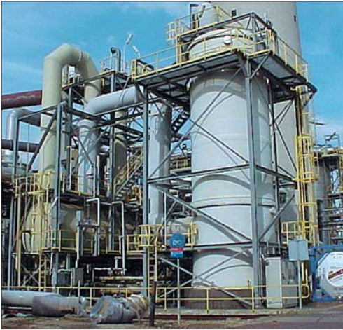
Fig. 34: Process plant made of vinyl ester resin
