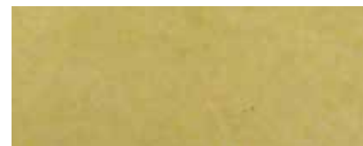
Cured resin, BPO/ Amine curing system
