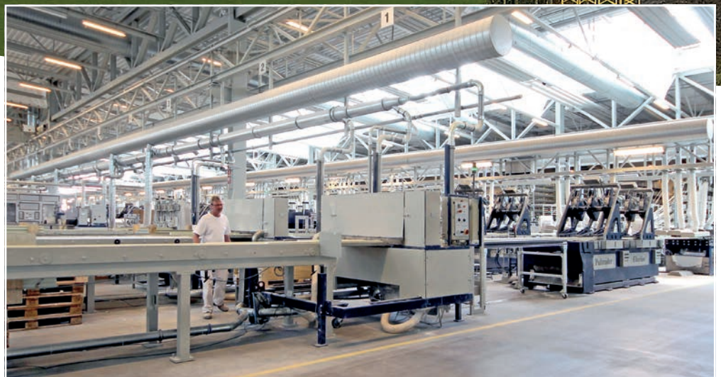
Industrial scale production of pultrusion profiles and panels (courtesy Fiberline Composites)
