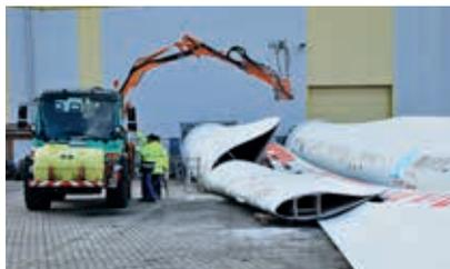
Mobile sawing equipment to reduce transport costs
