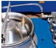
Safety valve in the container lid
