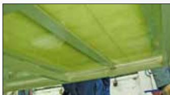
Preliminary tests to check drainage of the resin on the mould side draining
