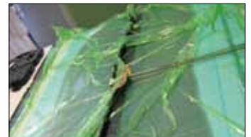
Drainage carried out with a peel ply and a PE flowing grid
