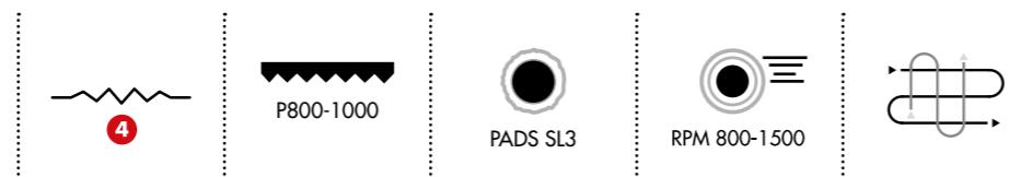
This is a super cutting compound especially recommended for applications on hard resins such as vinylester. It removes marks and P800-P1000 sand scratches very fast and well, according to the hardness of treated resins. It assures a high quality finish, without overheating and greasing the surface. NW 0 has been expressly formulated by our lab to serve the need of polishing the toughest moulds in the quickest way, achieving unbelievable results.
