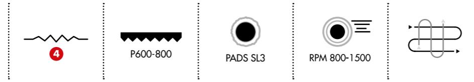
This is a super cutting compound used either to remove marks and P600-P800 sand scratches (according to the hardness of treated resins) or to restore high-oxidized gelcoats very fast and well, without overheating the surface. It assures a high quality finish without marks and haze as well as with low particles' oversplattering. NW 1 is widely appreciated as, through its specific abrasive components, it makes polishing easier and faster and allows to reduce the sanding processes.
