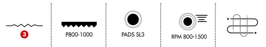
This is a medium cutting compound used either to remove marks and P800-P1000 sand scratches (according to the hardness of treated resins) or to restore oxidized gelcoats very fast and well, without overheating the surface. It assures an excellent gloss level, minimising the formation of holograms and minor marks. NW 6, through its perfectly balanced components, is the ideal solution for dark coloured and delicate surface treatment, where the aim is a first-class finish.
