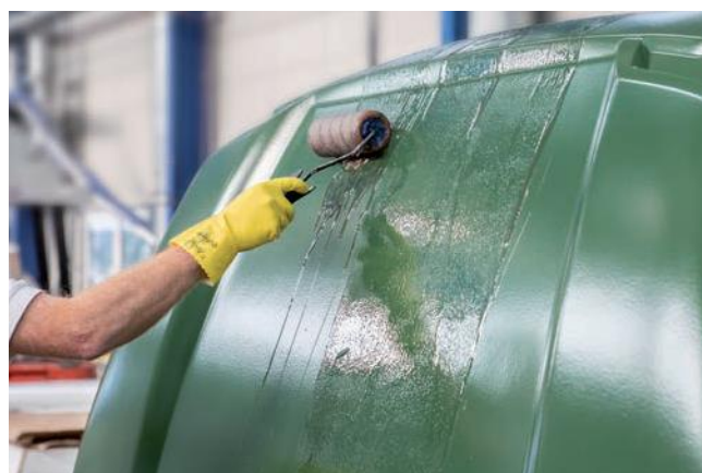
Application of first layer resin
