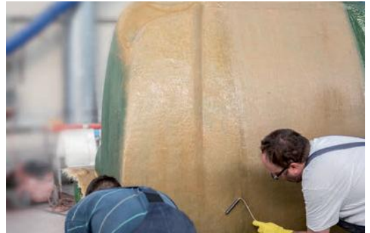
Applying mould-making resin
