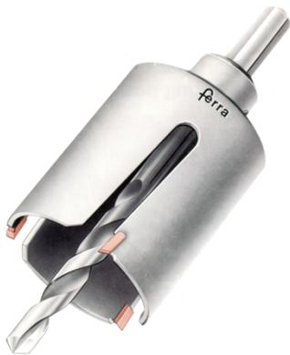
Plugs or large diameter holes can be cut-out even from higher density foam sheets with the help of special cutter cylinders. The numbers of bits are preferably kept low (for example about four). The use of hard-point tools is recommended. The cutting speed and feed-rate depends on the material characteristics and is best ascertained individually.
