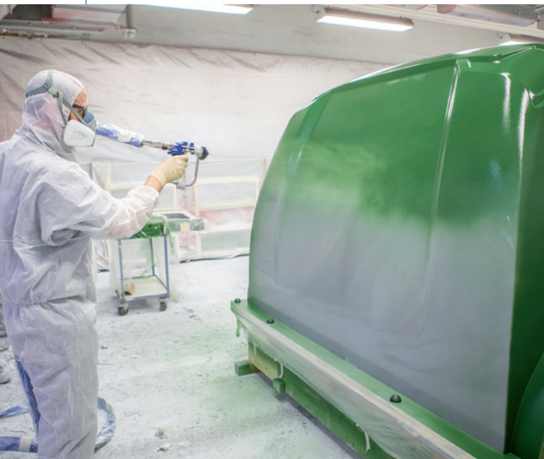
FIGURE 7 The components of the new Büfa mold-tooling system can be applied using conventional methods such as the spray-up process (example: gelcoat, left) and hand lay-up process (example: first-layer resin, right) (© Büfa)
