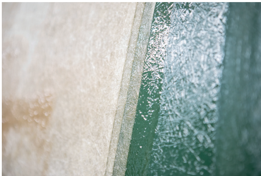
FIGURE 5 GRP parts made of unsaturated vinyl esters usually consist of several layers that are formed by specially designed resins; the surface quality is in part determined by the first-layer resin (© Büfa)
