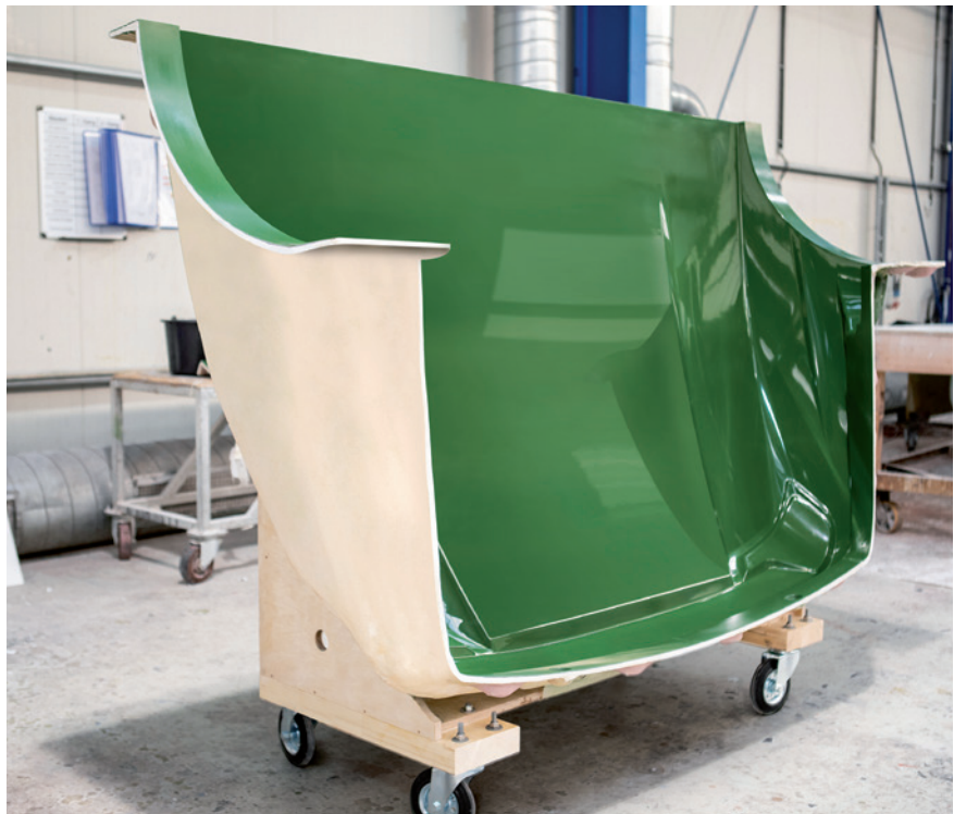
FIGURE 1 Dust accumulation caused by static electricity, and shrunken surfaces can be minimized thanks to the new, antistatic tooling system consisting of an antistatic gelcoat, an optimized first-layer resin and tooling resins (© Büfa)
