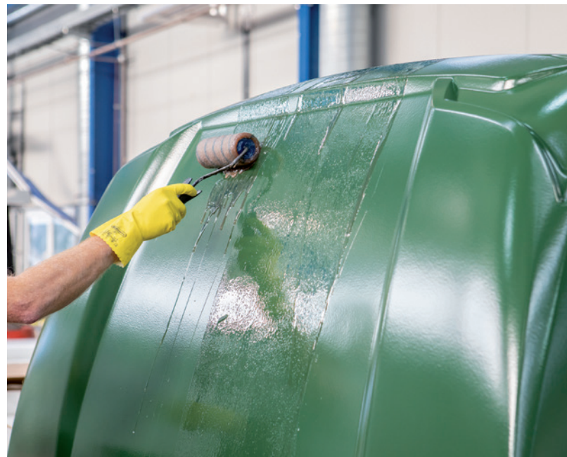
FIGURE 7 The components of the new Büfa mold-tooling system can be applied using conventional methods such as the spray-up process (example: gelcoat, left) and hand lay-up process (example: first-layer resin, right) (© Büfa)
