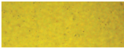
Cured resin, BPO/ Amine curing system
