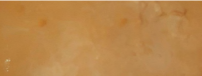
Cured resin, BPO/ Amine curing system
