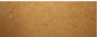
Cured resin, Standard MEKP/ cobalt curing system
