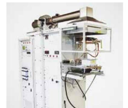
Cone calorimeter for investigating fire behaviour
